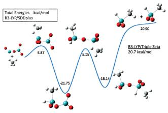
**Figure 11.** Reaction energy profile for the reaction of the 211 isomer of  $Mo_2O_4^-$  with two methanes.
