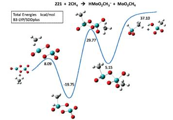
**Figure 12.** Reaction energy profile for the reaction of the 221 isomer of  $Mo_2O_5^-$  with two methanes.
