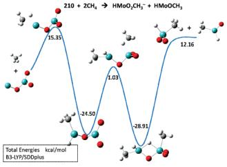
**Figure 9.** Reaction energy profile for the reaction of the 210 isomer of  $Mo_2O_3^-$  with two methanes.
